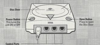
Use these ports to connect the Dreamcast Controller or other peripheral equipment. From left to right are Control Port A, Control Port B, Control Port C, and Control Port D. Use each port to connect controllers for players 1 to 4 respectively. NOTE: Control Port can also be referred to as Port.
