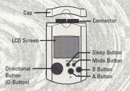
To automatically save score rankings, option settings and other game information, insert a Visual Memory Unit (VMU) into Expansion Slot 1 of the controller in Control Port A BEFORE turning on the Sega Dreamcast.
