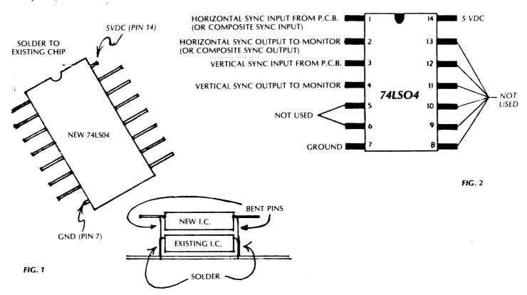
CURE 2: Used for Wells-Gardner Video-Sync boards with positive sync connections only. (Vertical mount board 85x14 OB.
