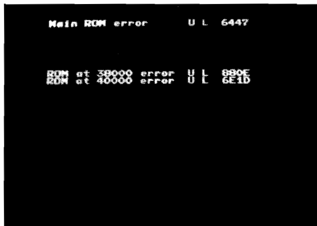
Figure 3-2 ROM Test Fails
