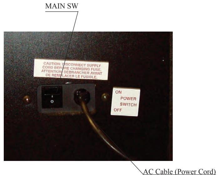
FIG. 6. 3 b AC UNIT OF THE MAIN PROJECTION UNIT
