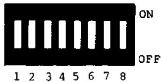
FIGURE 1, 8-Position DIP Switch
