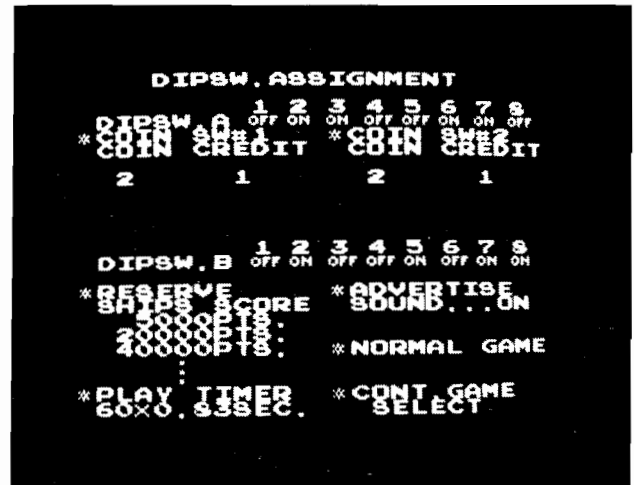
Self-Test - Dip Switch Assignment
